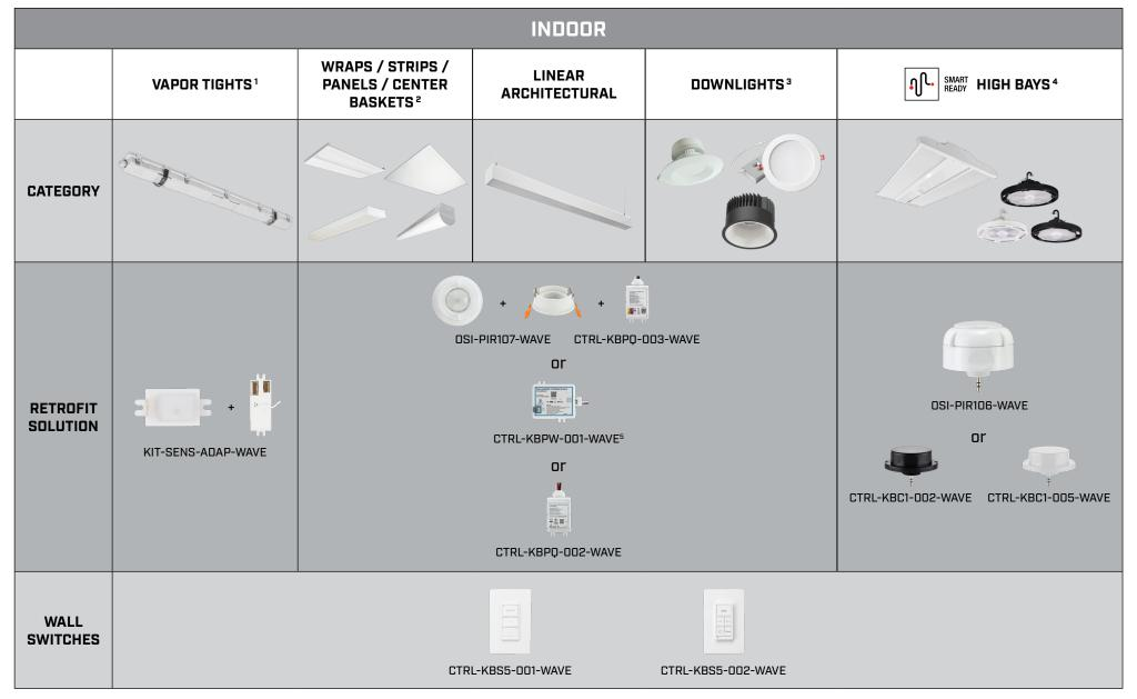
**General note:** The Wave Smart accessories are compatible with 0 - 10 V dimming only.
