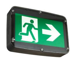
The RPN series of wet location anti vandal running man is designed to operate in extreme environments. The unit, designed using a polycarbonate housing, maintains its sealed interior with a continuous integral gasket. As well, LED pilot light and test switch are sealed type. Available in AC/DC and internally self-powered versions.
