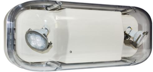
The EBNX series of battery units is designed to operate in the most extreme environments. The unit, designed using a polycarbonate housing, maintains its sealed interior with a continuous integral gasket. The EBNX series is available in 6 V DC and 12 V DC versions in 36 W, 50 W, 72 W, 100 W or 130 W wattage capacity for a minimum of 30 minutes in emergency mode. Auto test feature is standard.
