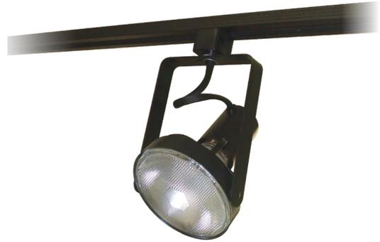
Front loaded economical PAR38 Gimbal style track head. Integral on/off switch and track polarity indicator come standard. The AG05N comes complete with J & J2 style track adapter. H & H2 style adapter available upon request. Suitable for ceiling-mounted tracks.
