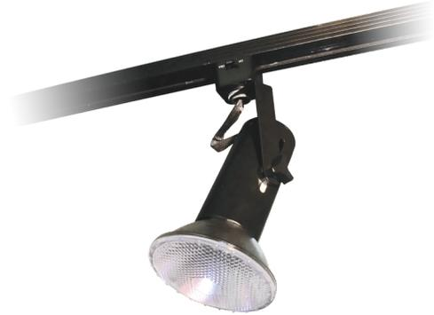
The economical adjustable socket style track head allows for the proper seating of various lamps. Integral on/off switch and track polarity indicator come standard. The AL10 comes complete with J & J2 style track adapter. Suitable for ceiling-mounted tracks.
