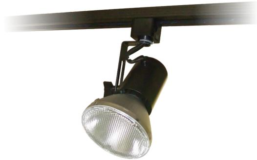
The economical adjustable side swivel track head allows for the proper seating of various lamps including PAR30 long neck. It features a half yoke design with slide adjustment slot to maximize the fixture height options. Integral on/off switch and track polarity indicator come standard. The AL95 comes complete with J & J2 style track adapter. Suitable for ceiling-mounted tracks.
